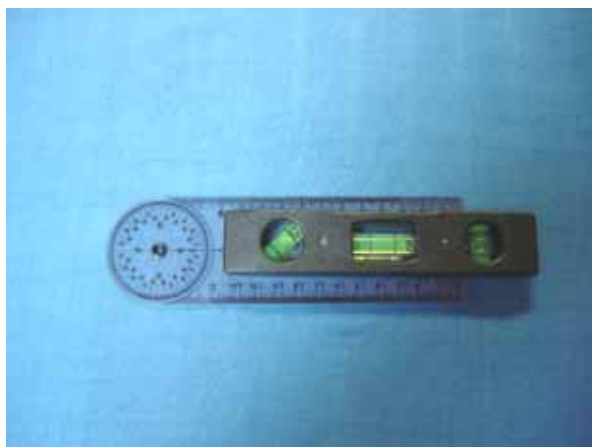
Fig. 2 Protractor for measuring shoulder slope
