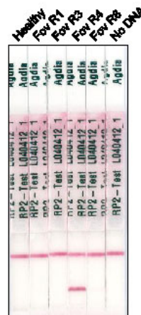
AmplifyRP strips showing the detection of Fov R4 in cotton by AmplifyRP nfo assay
