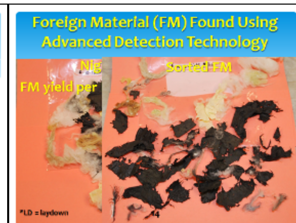
Figure 8. FM Found Using Advanced Technology
