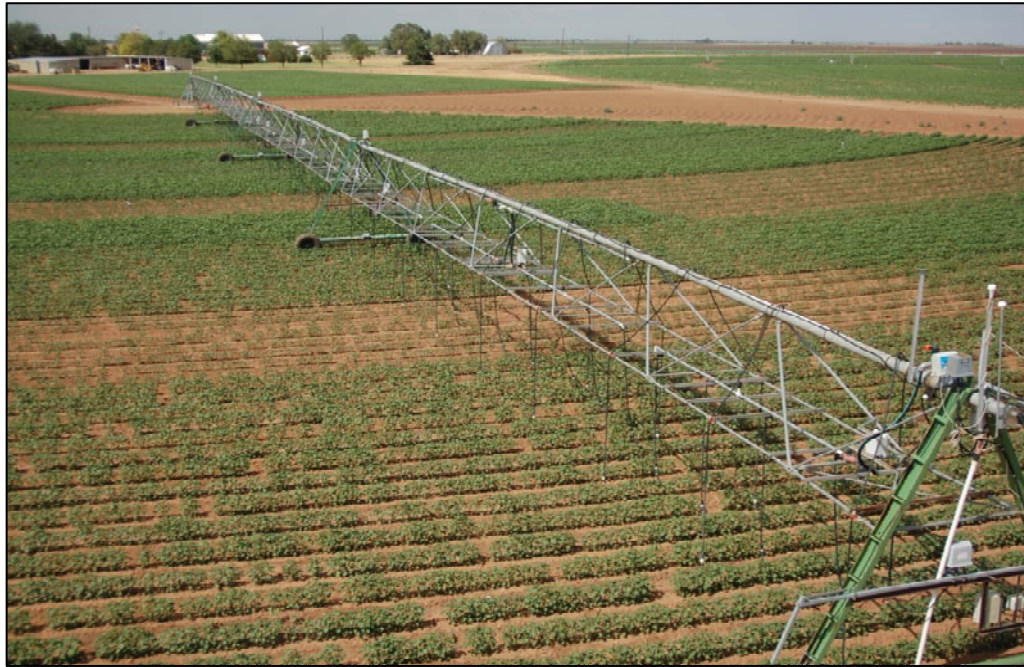
Figure 3. Site-specific LEPA irrigation system used to water three replicates of 27 different irrigation treatments in experiments conducted at the Texas A&M AgriLife Research Center at Halfway, 2010-2012.
