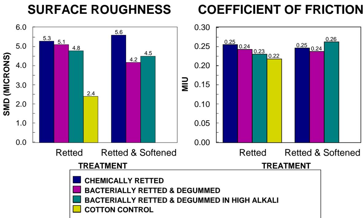
**Figure 3. Fabric surface friction as evaluated with the Kawabata system.**
