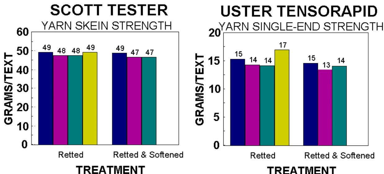
Figure 2. Yarn strength as measured with strength tester (Scott) and Tensorapid (Zellweger Uster).
