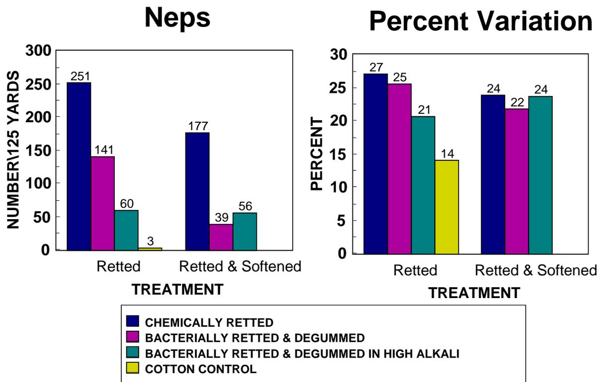
Figure 1. Yarn uniformity as measured with evenness tester from Zellweger Uster.
