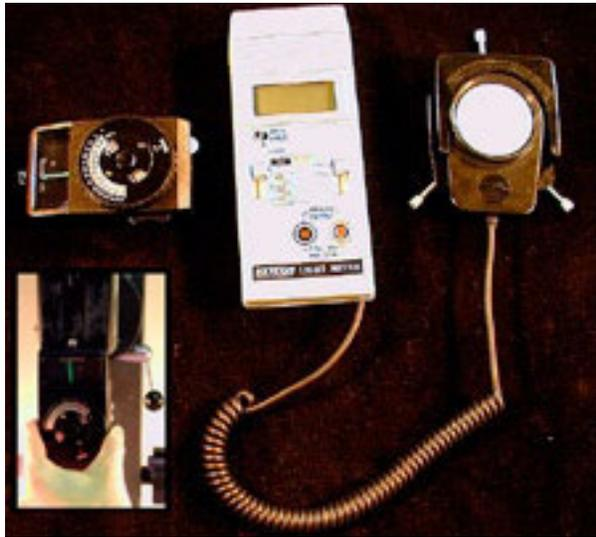
Figure 4: Consistent images are produced for analysis by using reflective measurements as a tool to adjust lighting. Aiming the Vivitar 45 Exposure meter towards the fabric with ASA set at 800, the rheostat was used to adjust the lights until the meter read 11 EV to set the level of lighting. The lighting was fine tuned using the An Extech Instruments digital light meter (Model 401025).
