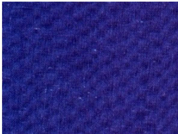
Figure 1: Dyed fabric displaying white specks.
