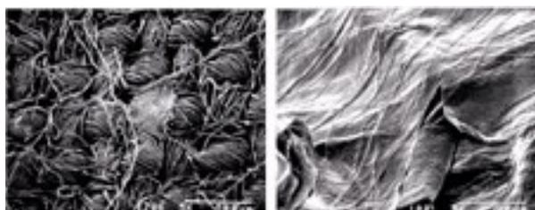
**Figure 2: Photomicrographs of white specks on a dyed fabric.**
