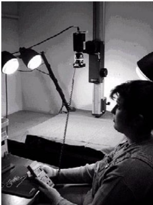
Figure 5: The lighting was fine tuned using a digital light meter (Model 401025). The rheostat was adjusted until the light meter luminance reading was  $198^{\circ}2 \text{ lm/m}^2$  ( $198^{\circ}2 \text{ Lux}$ ).
