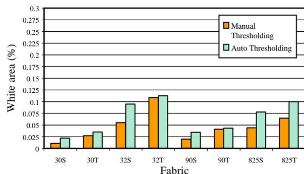
**Figure 7: Comparison of manual and auto thresholding. Maximum foreground set to 20% for normal and high white speck fabrics (32S, 32T, 90T, 825S, and 825T) and to 10% for low white speck fabrics (30S, 30T, and 90S).**
